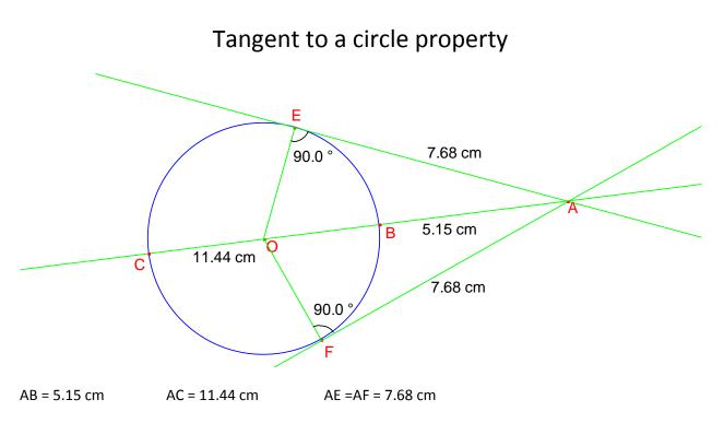
Now check that AE x AF = AB x AC (Note: due to measurement errors the equality is only approximate)
